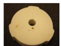
Successful compacted and sintered part
