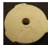
Part with Crack
