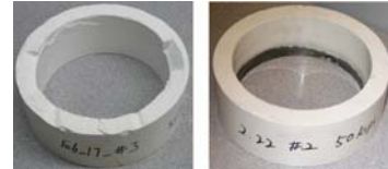
Unsuccessful and successful formed green parts
