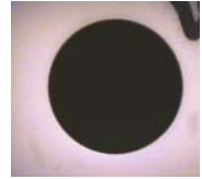
Exit of the Hole, Drilled by Improved Core Drill on CNC Machine
