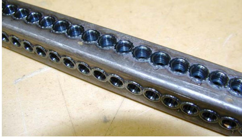
Figure 5.4. Close up view of square tube workpiece after friction drilling tool wear test.
