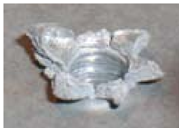
Figure 1.6. Friction drilling cast Al part with flower shape bushing.
