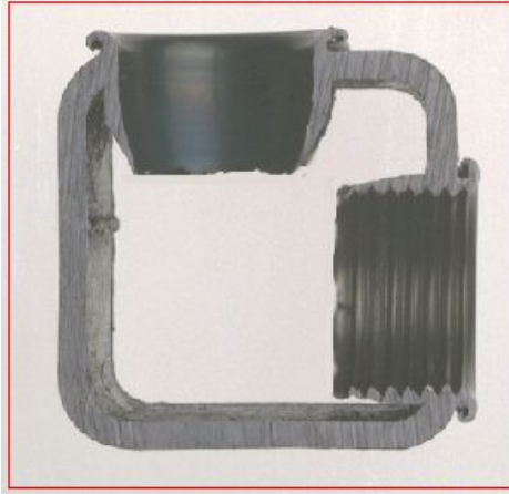
Figure 1.2. Resulting hole and bushing [19].
