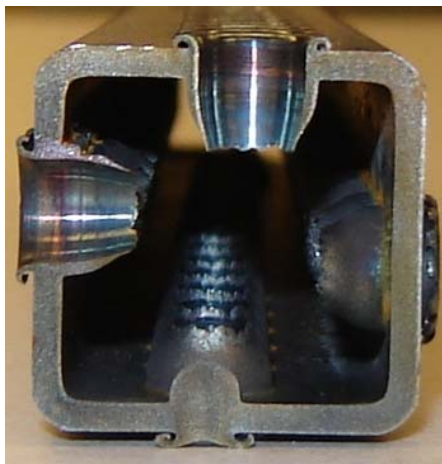
Figure 5.2. Cross section of friction drill holes in AISI 1015 steel tube.
