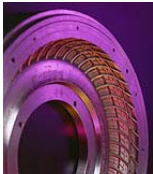
Fig. 1.2. An example of the mold used for tire tread pattern molding.
