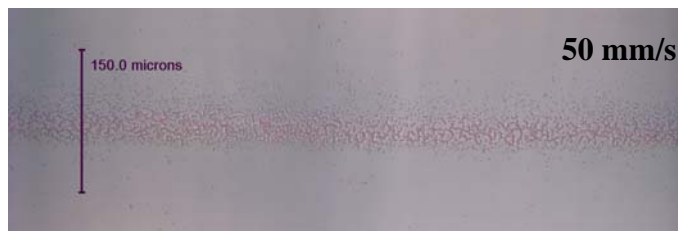
Figures 31 - 33: Lines written at 5, 25, and 50mm/s speed
