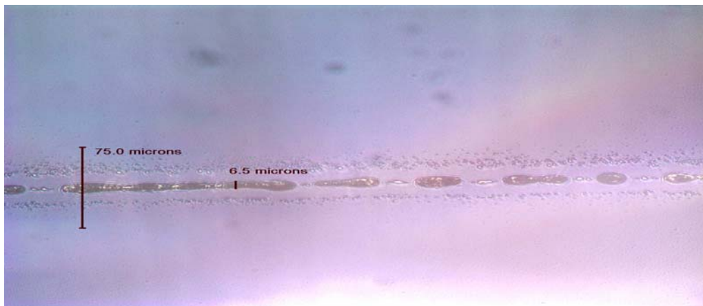
Figure 20: Clumping of particles due to high solids content.
