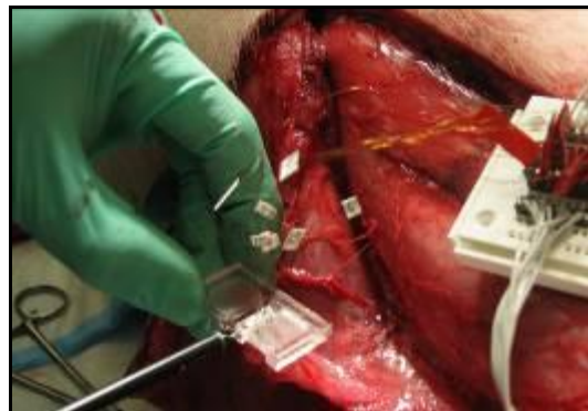
Figure 9. Experimental setup showing surgical tool, fixture, and thermistors.
