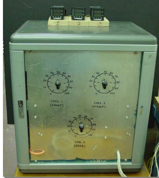
Figure 4.6: Blackbody radiation source power, solid-state relay, and controller housing.
