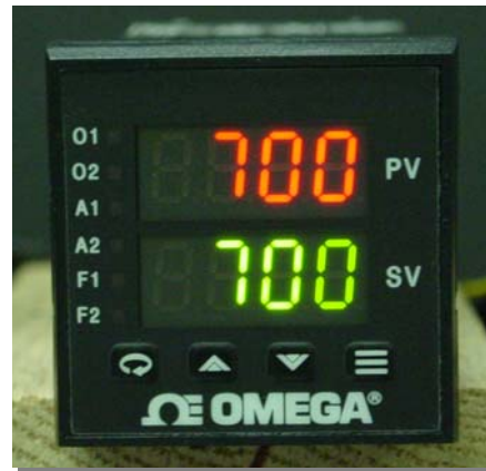
Figure 4.7: Omega PID controller used with Inconel blackbody. PV=process value, SV= set value
