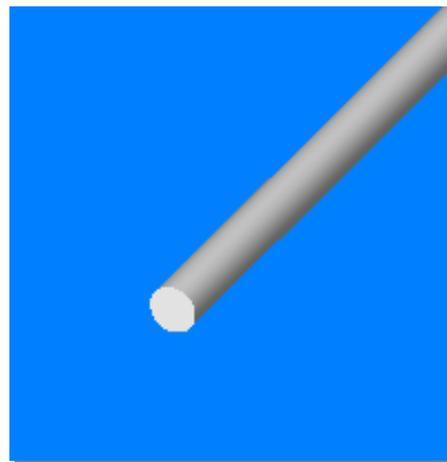
*Figure 1.1: Flat tip optical fiber.*
