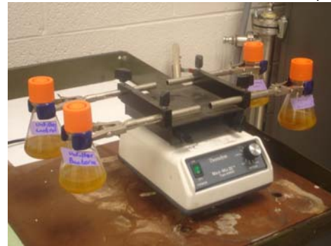
Samples in 9K media were agitated in vented flasks. (Apparatus is shown at left)
